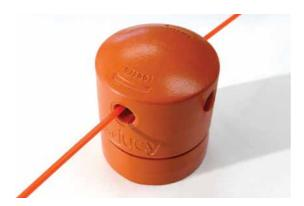
line. The parts fasten together on a large thread which enables the top part of the head to be easily adjusted 90 degrees for insertion of new nylon; rotation of the trimmer head tightens the strips of nylon line within the assembly during use.
